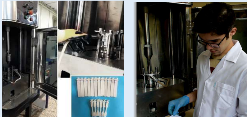
Injection molding sample fabrication based on the ASTM standards
